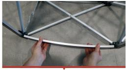
6. Place the long curved bars horizontally on the frontside of the frame.
