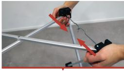
2. Push the hinges towards each other and lock the frame by connecting the metal hooks.
