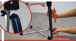
**4.** Insert the pointed topside of the bar in the groove. **5.** Lift slightly and slide in the bottom side of the bar.
