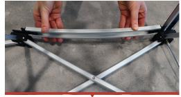
Place the short curved bars horizontally on the backside of the frame.
