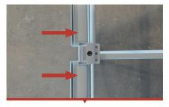
Slide in the aluminium bars from the side, on both the front and the backside of the frame.
