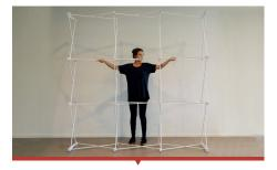
**4.** Gently lift up the frame while flipping it over, the pop-up frame will unfold itself.
