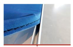
**9.** Attach the fabric by pushing the silicone edges in de grooves.
