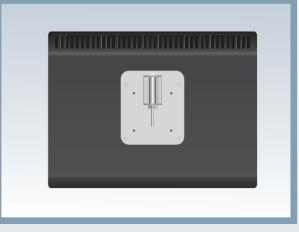
Screw the fastening plate on the back of the screen. Fits VESA standard 70 and 100
