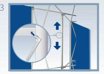
Adjust, with the help of an Allen key, the horizontal stay so that it fits the hole that you have made in the panel. Put the graphic panel back into place.
