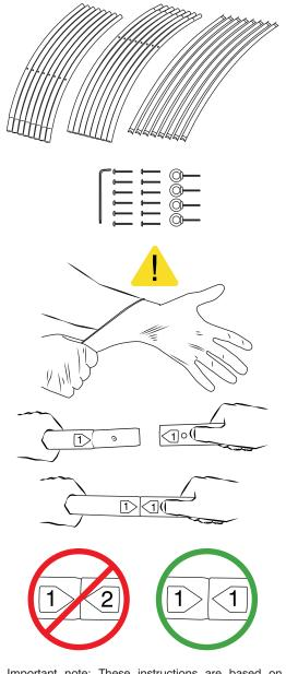
Important note: These instructions are based on assembling the 3m version. Other size kits will have slightly different configurations of poles but can still be assembled in the same way.
