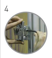
Adjust and tighten 4 screws at side of Interface bracket until securely clamped to post in desired position.
