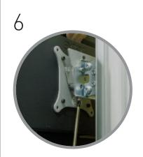
Insert screw up through bottom centre of assembled bracket and monitor mount, and tighten to secure monitor in place.
