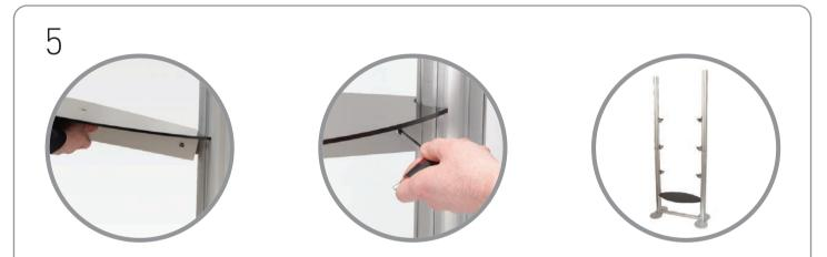
With the black acrylic uppermost, slide first assembly into the same post channels as the bottom profile, until the expanding clamps rest on the pre-installed locator bars of the bottom posts. Tighten grub screws in ends of profile to secure in position.
